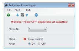
• If more than one STC 816 R/PSU 8-16 R are connected via a management unit, select an individual head-end station via pull down menu "Station No.".
