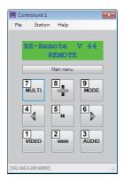
Via this menu the control unit of the plant can be remote controlled. If several stations are connected select the corresponding control unit in menu "Station". The keys of the figure are designed as buttons (mouse control).
