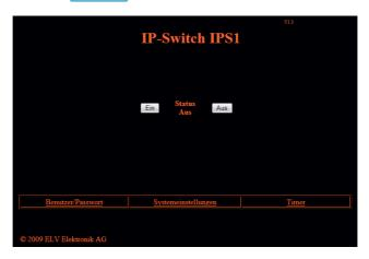
Via buttons **Ein** (on) and **Aus** (off) you can change the switching status of IPS1.
