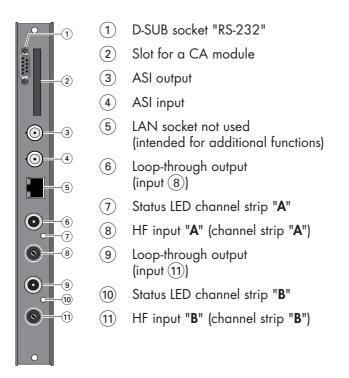
The operating software of the cassette can be updated via the 9-pin D-SUB socket "RS-232" using a PC or notebook and the software "**BE-Flash**". You can find the current operating software on the website "**www.gss.de**".
