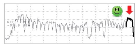
Graph the spectrum which is present at the device output 10 with a measuring instrument and equalize the output level of the "new" transponder to the spectrum.
