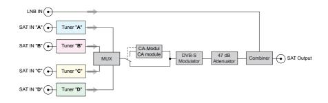
The 4 tuners receive their input signal from the outputs of a multiswitch. If no further input is free for the converted signal at the multiswitch, the corresponding satellite band can be multiplexed with the converted signal via the LNB input and then feed into the multiswitch. There are two fields of application for the device:
