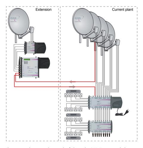
The converted transponder must be fed into the SAT IF range with the same frequency range.
