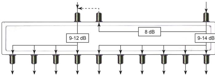
Unused loop-through outputs must be terminated with the resistors supplied. The power supply in the head-end station is designed to supply power to components (e.g. LNBs) connected upstream. These are supplied via the SAT IF input distributors' input sockets with operating voltage (+18 V) at a total current of max. 1 A ==.
