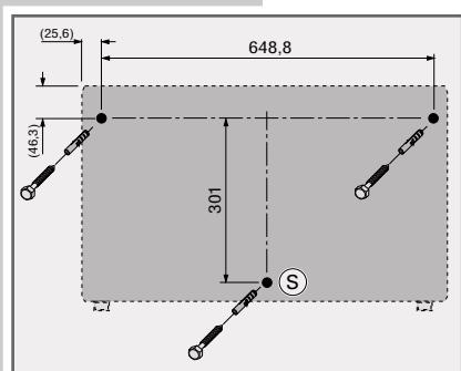
1 Fix the screws according to the Figure, and then hook in the professional satellite unit (ensure a flat surface!).
