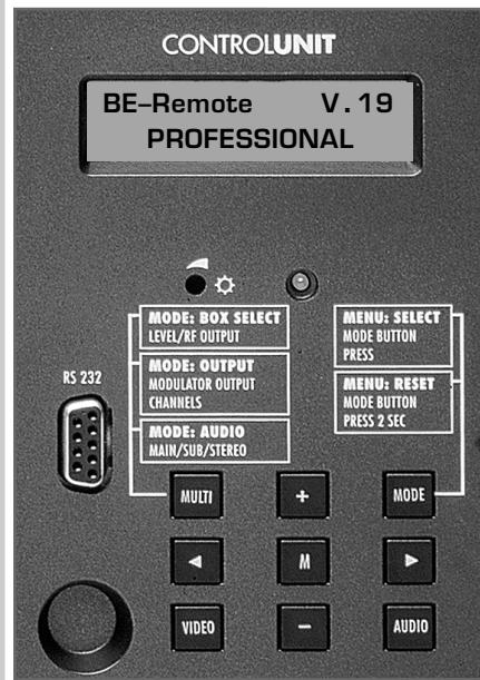
All input and outputs parameters of the individual boxes can be selected with the keys on the control panel.
