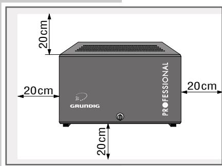
Therefore never cover the bottom and top ventilation slots in the housing. If several units are installed on top of each other or side by side, minimum distances of 20 cm must be kept in all directions.
